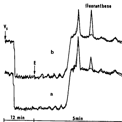
Fig. 2. Determination of fluoranthene in tap water (city of Brno). Mixer, analytical column and precolumn, see Fig. 1. Sampling: 200 \mu\text{l} of water in 45% methanol into the precolumn. Desorption from the precolumn: 19 \mu\text{l} of methanol. V_s = sampling of 14 \mu\text{l} of methanolic extract and 15 \mu\text{l} of distilled water into the mixer and analytical column. E = elution with 90% methanol, flow-rate 5 \mu\text{l}/\text{min} . Water analysis (a) without addition of fluoranthene, concentration determined 120 ng/l; (b) with addition of fluoranthene (100 ng/l). Dotted line indicates blank.
